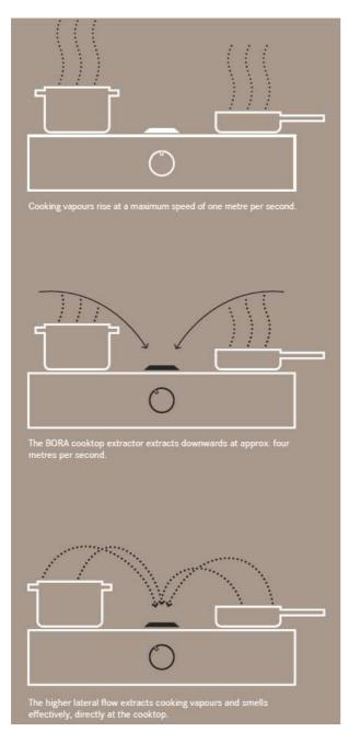
BORA stops cooking vapours and odours from rising in the first place by extracting them from the place they are created. The concept is based on applied physics and the basic principles of fluid mechanics: the lateral flow is greater than the rising speed of the cooking vapour from pots and pans. From a purely physical perspective, it is therefore easier to directly extract the vapour at the cooktop.
