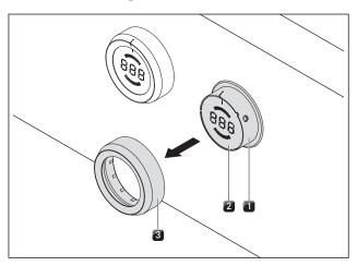
Fig. 7.5 Pull out the knob ring
