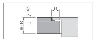
Fig. 5.4 Groove dimensions for flush installation
