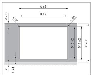
Fig. 5.3 Cut-out dimensions for flush installation
