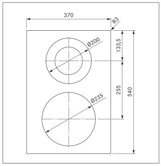
Fig. 3.2 PKCH2 Device dimensions aerial view
