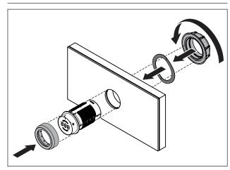
Fig. 5.10 Fitting the control knob
