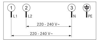
Fig. 5.23 Connection diagram 2-phase
