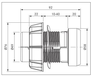
Fig. 3.1 Device dimensions control knob
