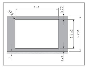
Fig. 5.5 Cut-out dimensions for surface mounting
