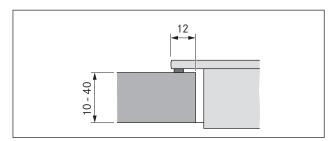
Fig. 5.6 Surface mounting cut-out
