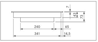
Fig. 3.3 PKCH2 Device dimensions front view
