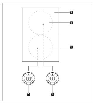
Fig. 5.20 Standard cooking zone connection
