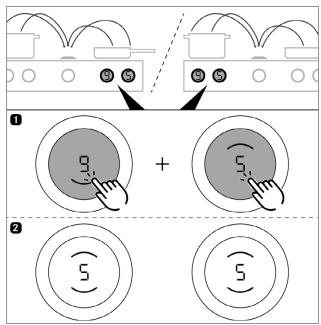
Fig. 5.26 Activating the bridging function
