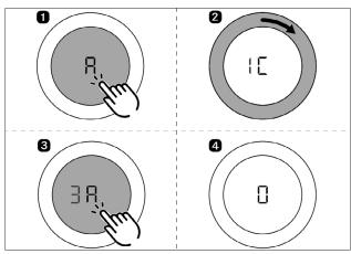
Fig. 5.16 Deactivating the automatic extractor function
