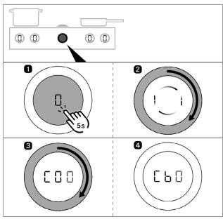
Fig. 6.5 access the configuration menu
