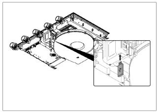
Fig. 6.3 Inserting the USB stick
