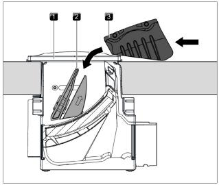
Fig. 7.3 Fitting the cover flap
