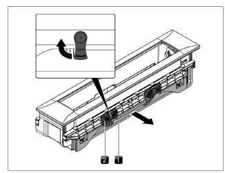
Fig. 7.4 Removing the maintenance tray
