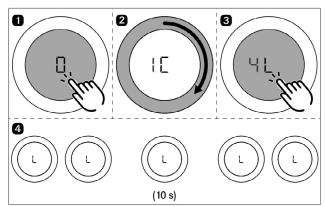
Fig. 5.17 Permanently activating the child lock
