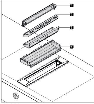
Fig. 3.7 Filter components
