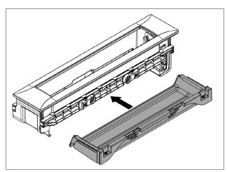
Fig. 7.5 Installing the maintenance tray
