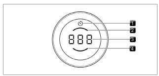
Fig. 3.3 Control knob display elements
