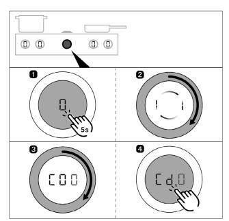
Fig. 6.8 Checking the software version
