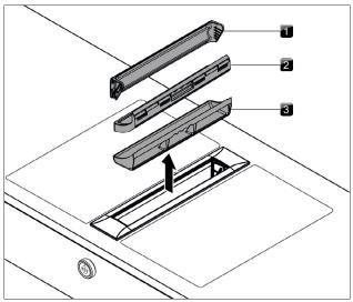
Fig. 7.1 Removing the grease filter components
