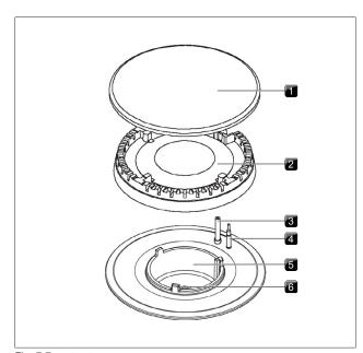
Fig. 7.7 Gas burner structure
