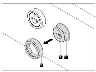
Fig. 7.8 Pull out the knob ring
