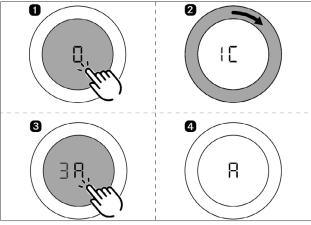
Fig. 5.15 Activating the automatic extractor function
