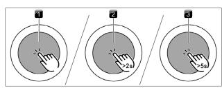
Fig. 5.2 Diagram of the touch commands
