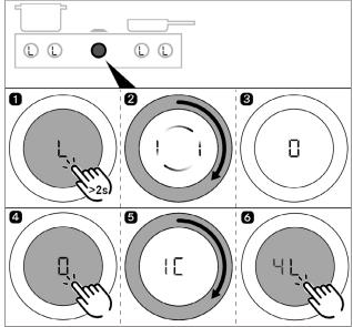
Fig. 5.19 Permanently deactivating the child lock
