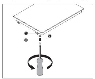
Fig. 5.16 Mounting brackets
