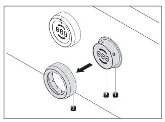
Fig. 7.5 Pull out the knob ring
