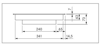
Fig. 3.2 PKC32 Device dimensions front view
