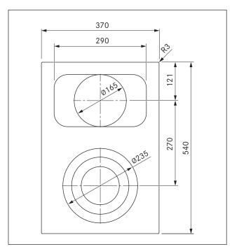
Fig. 3.4 PKC3B Device dimensions aerial view
