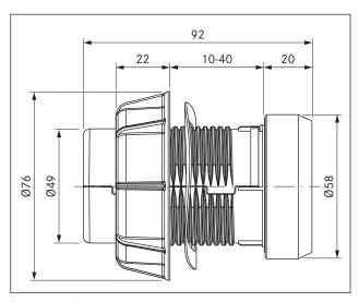
Fig. 3.7 Device dimensions control knob
