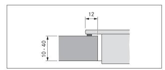
Fig. 5.6 Surface mounting cut-out
