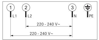
Fig. 5.23 Connection diagram 2-phase
