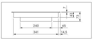
Fig. 3.5 PKC3B Device dimensions front view
