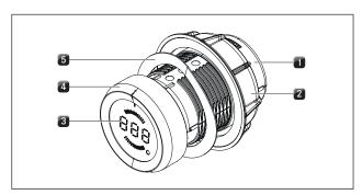
Fig. 4.3 Structure of control knob
