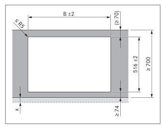
Fig. 5.5 Cut-out dimensions for surface mounting
