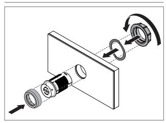
Fig. 5.10 Fitting the control knob
