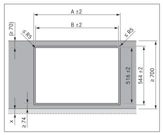
Fig. 5.3 Cut-out dimensions for flush installation
