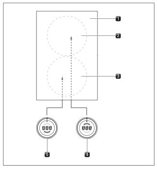
Fig. 5.20 Standard cooking zone connection
