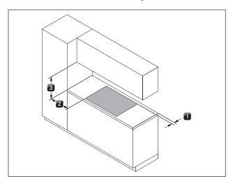
Fig. 5.17 Minimum clearances for installation rotated by  $180^{\circ}$
