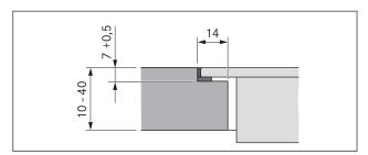
Fig. 5.4 Groove dimensions for flush installation
