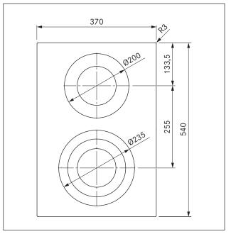
Fig. 3.1 PKC32 Device dimensions aerial view
