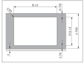
Fig. 5.5 Cut-out dimensions for surface mounting
