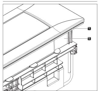
Fig. 5.7 Removing the plastic bar from the cooktop extractor
