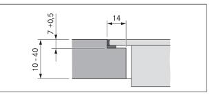
Fig. 5.4 Groove dimensions for flush installation
