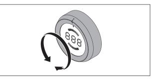
Fig. 6.2 Switching on the cooking zone
