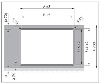
Fig. 5.3 Cut-out dimensions for flush installation
