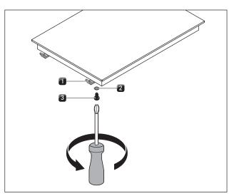
Fig. 5.19 Mounting brackets
