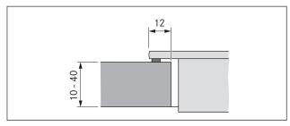
Fig. 5.6 Surface mounting cut-out
