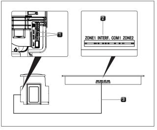
Fig. 5.22 Connection of the automatic extraction system
