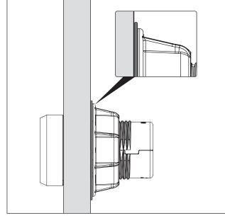
Fig. 5.14 Wave spring once assembly is complete
