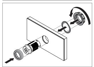
Fig. 5.13 Fitting the control knob
