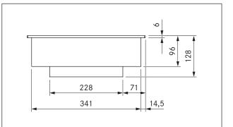
Fig. 3.3 PKIW1 Device dimensions front view
