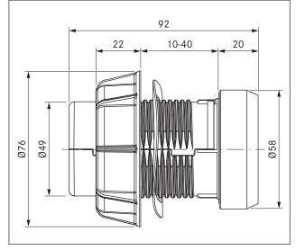
Fig. 3.1 Device dimensions control knob
