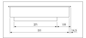
Fig. 3.4 PKIW1 Device dimensions side view
