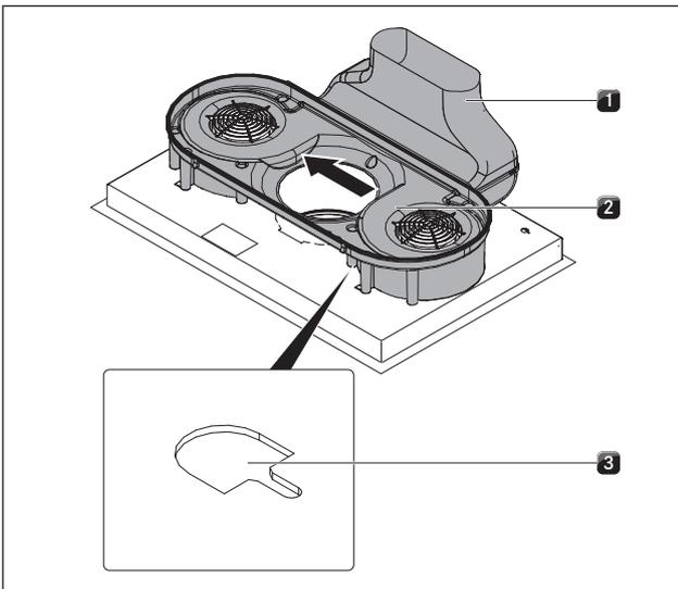
Fig. 6.26 Moving the air guiding housing
