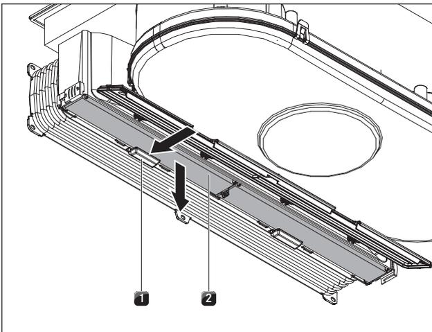
Fig. 8.8 Removing the activated charcoal filter
