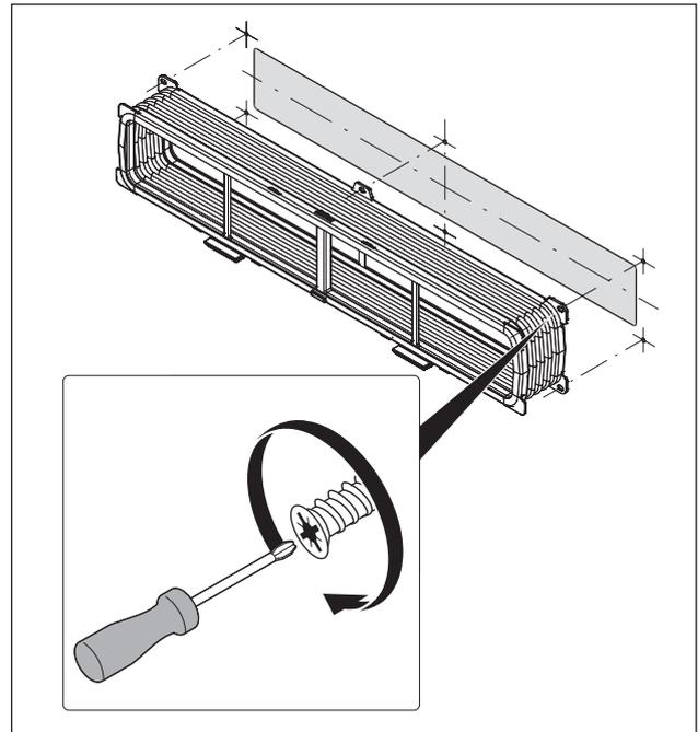
Fig. 6.12 Flexible duct with 6 EURO screws 6.3x10 mm
