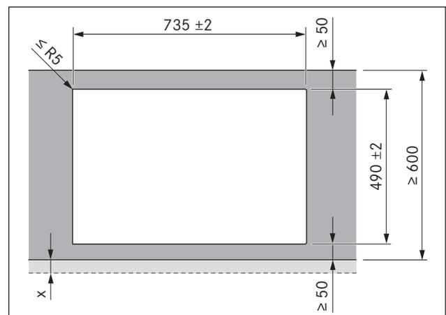
Fig. 6.5 Dimensions of cut-out for surface installation
