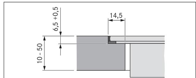
Fig. 6.4 Dimensions of groove for flush installation
