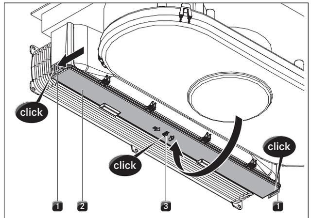
Fig. 8.10 Closing the activated charcoal filter housing cover
