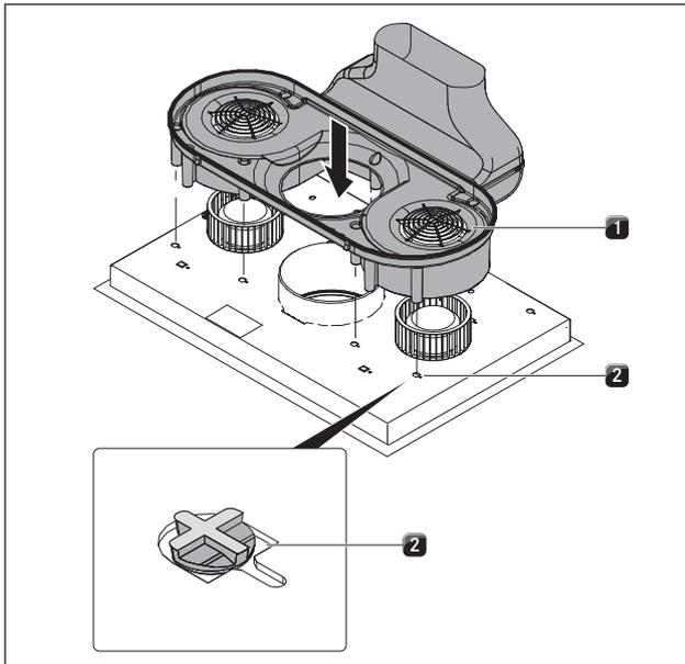
Fig. 6.30 Inserting the airflow assembly on the cooktop base
