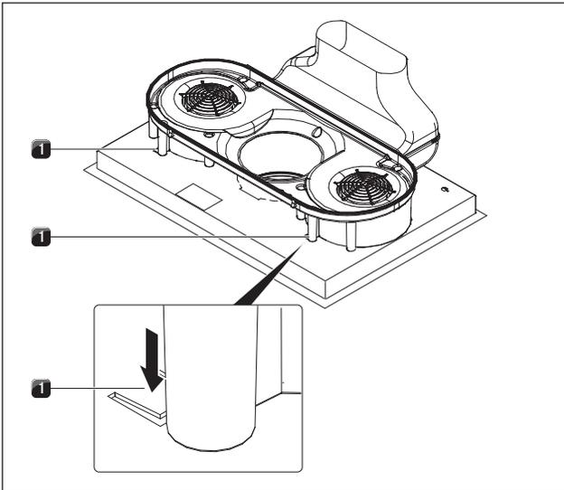
Fig. 6.25 Releasing the position lock
