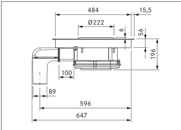
Fig. 3.4 Device dimensions with cable extension (BIA + BLAVH1)
