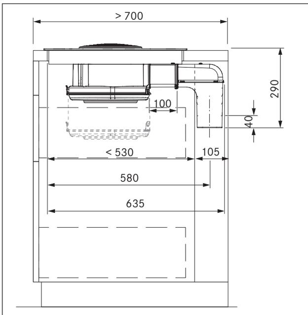
Fig. 6.23 Installation dimensions for exhaust air, worktop depth 700 mm
