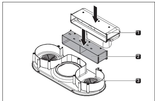
Fig. 6.29 Inserting the extension for exhaust air duct
