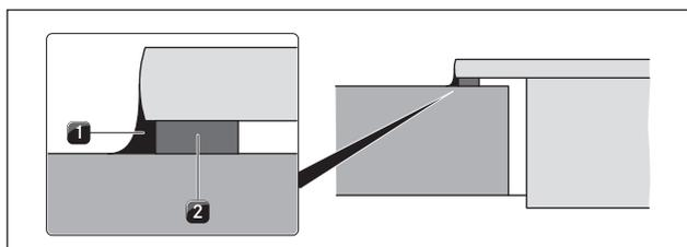
Fig. 6.7 Sealing tape, surface installation
