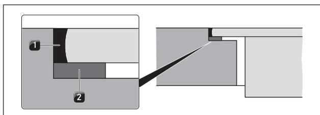
Fig. 6.8 Sealing tape, flush installation
