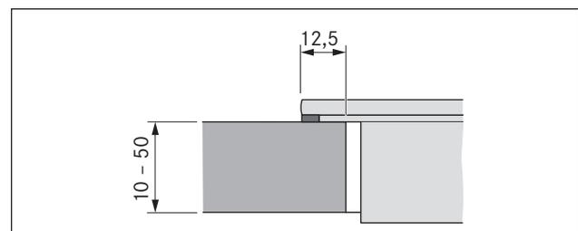
Fig. 6.6 Dimension of support for surface installation
