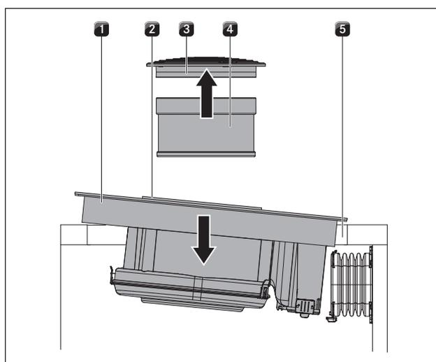
Fig. 6.13 Insert the cooktop at an angle
