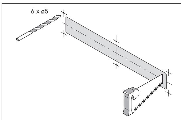
Fig. 6.11 Cut-out and connection bores
