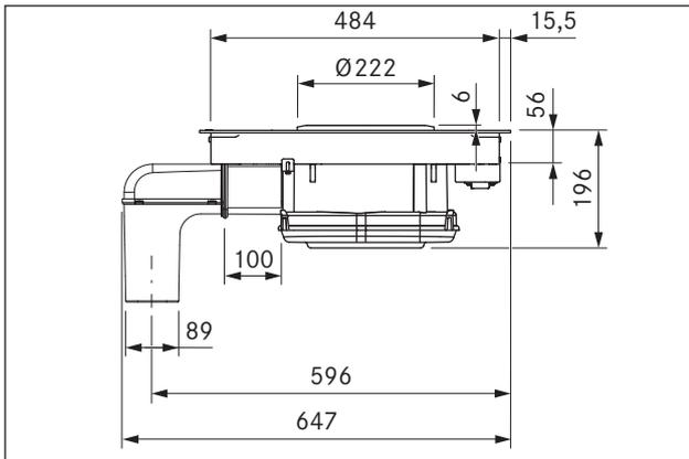
Fig. 3.4 Device dimensions with cable extension (BHA + BLAVH1)
