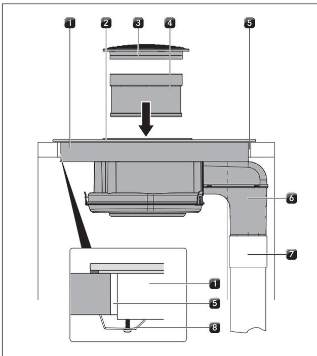
Fig. 6.35 Connecting the exhaust air duct + secure
