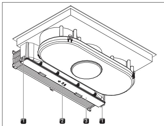
Fig. 8.5 Releasing the activated carbon filter housing lid
