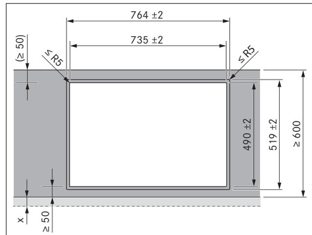
Fig. 6.3 Dimensions of cut-out for flush installation
