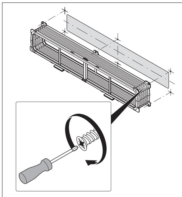
Fig. 6.12 Flexible duct with 6 EURO screws 6.3x10 mm
