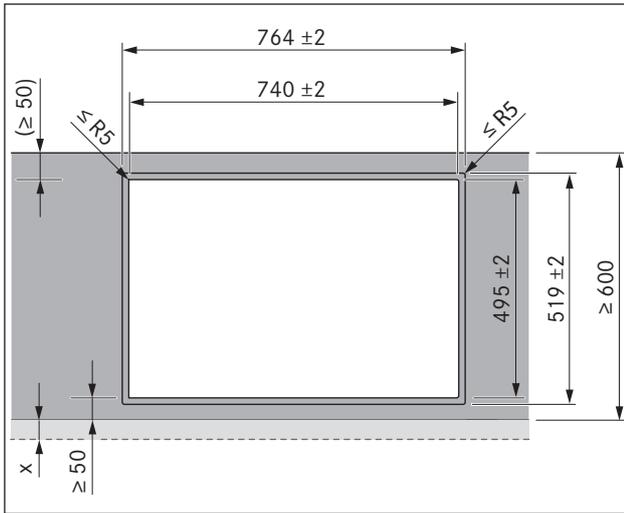
Fig. 6.4 Cut-out dimensions for flush installation
