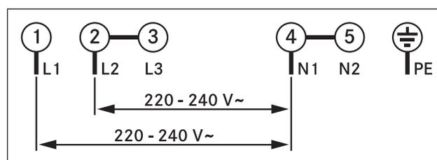
Fig. 6.34 Connection diagram 2-phase connection
