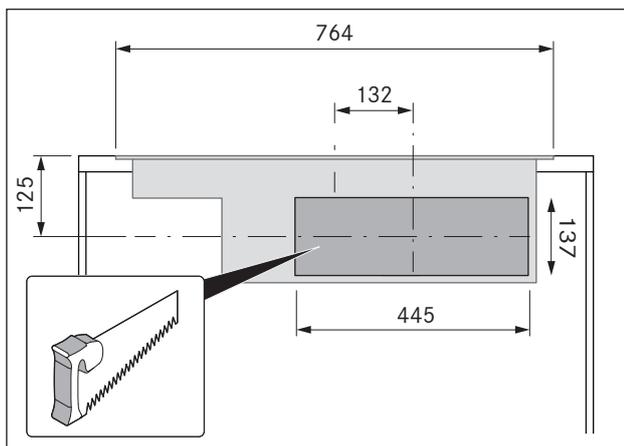
Fig. 6.11 Cut-out for return flow aperture
