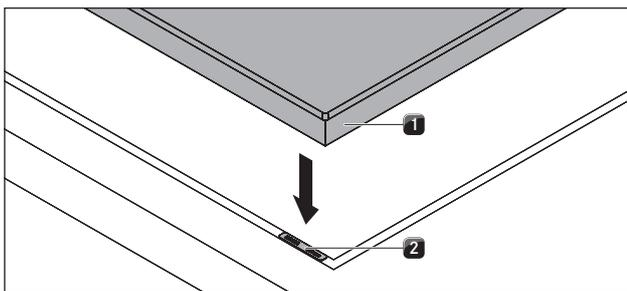
Fig. 6.15 Height adjustment plates
