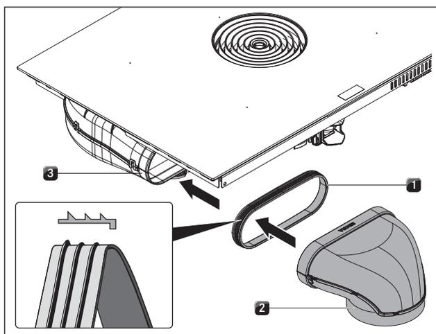
Fig. 6.32 Connecting the duct system
