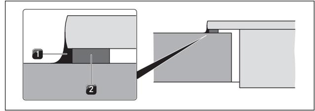
Fig. 6.8 Sealing tape in surface mounting
