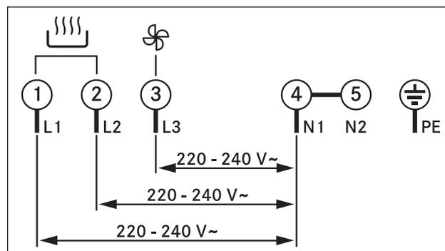
Fig. 6.33 Connection diagram 3-phase connection
