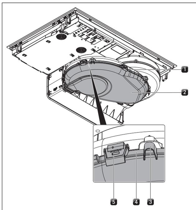
Fig. 8.3 Air guiding housing
