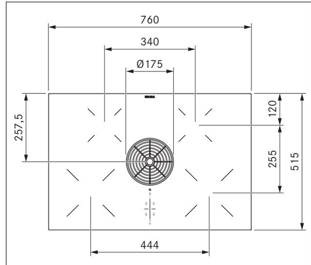
Fig. 3.1 PURA device dimensions top view
