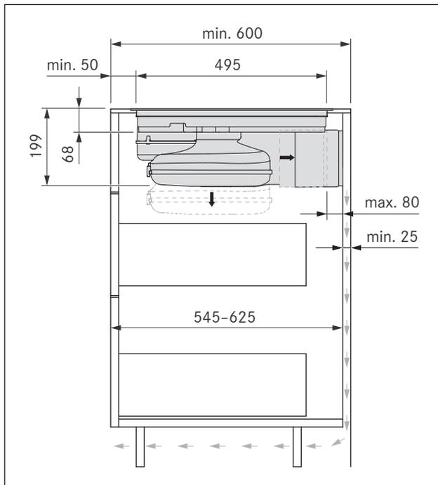
Fig. 6.10 Installation dimensions for recirculation, depth of worktop 600 mm
