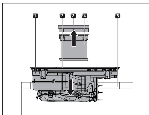
Fig. 6.28 Inserting the cooktop
