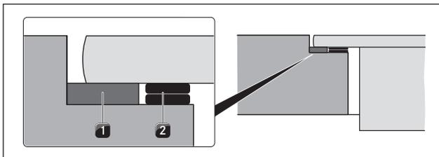
Fig. 6.30 Height adjustment plates
