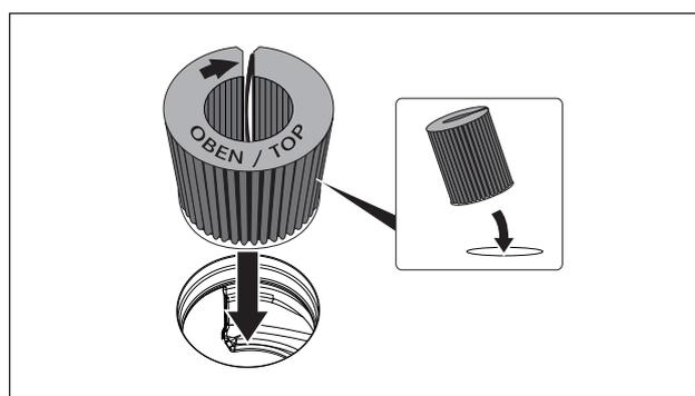
Fig. 6.21 Inserting the activated charcoal filter through the vent opening
