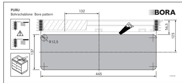
Fig. 6.12 Template for back wall cut-out
