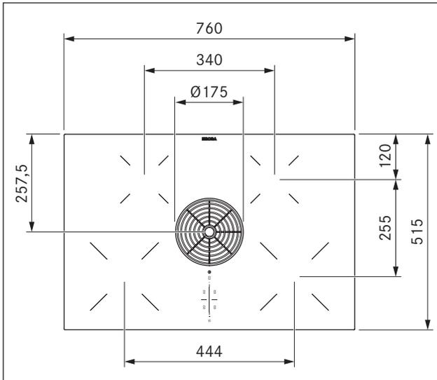
Fig. 3.4 PURU device dimensions top view
