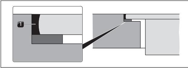
Fig. 6.41 Silicone sealant in flush installation
