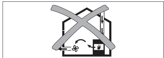
Fig. 6.24 Exhaust air installation - not permitted
