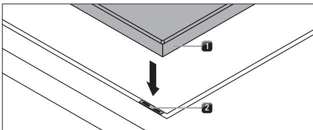
Fig. 6.29 Inserting height adjustment plates
