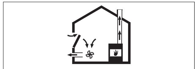
Fig. 6.25 Exhaust air installation - correct
