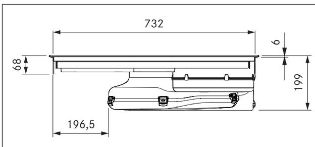
Fig. 3.5 PURA device dimensions front view
