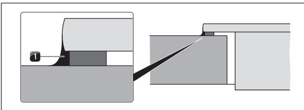
Fig. 6.42 Silicone sealant in surface mounting
