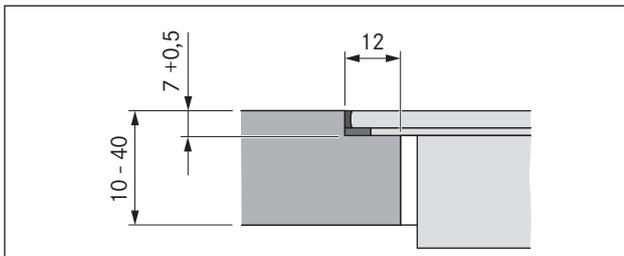
Fig. 6.5 Rebate dimensions for flush installation
