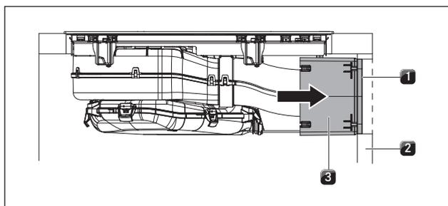
Fig. 6.18 Connecting the telescopic duct to the back wall
