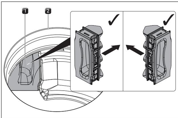
Fig. 6.23 Inserting the filter replacement cover
