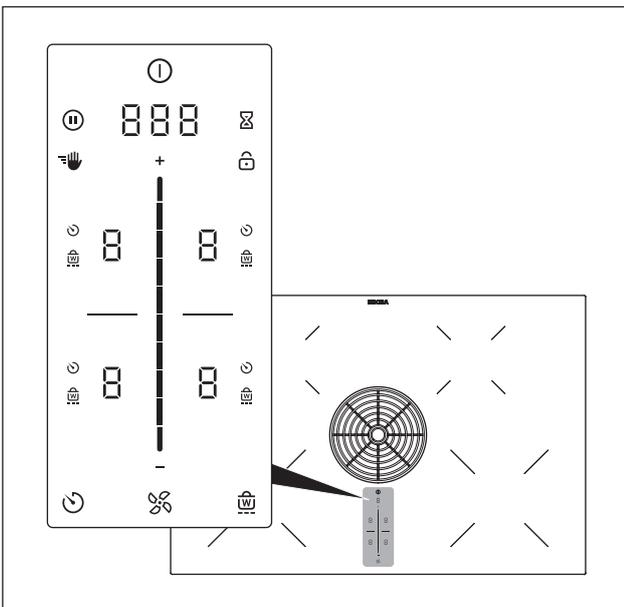
Fig. 5.4 Central touch/slider operating panel
