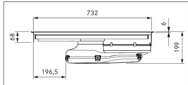
Fig. 3.2 PURA device dimensions front view
