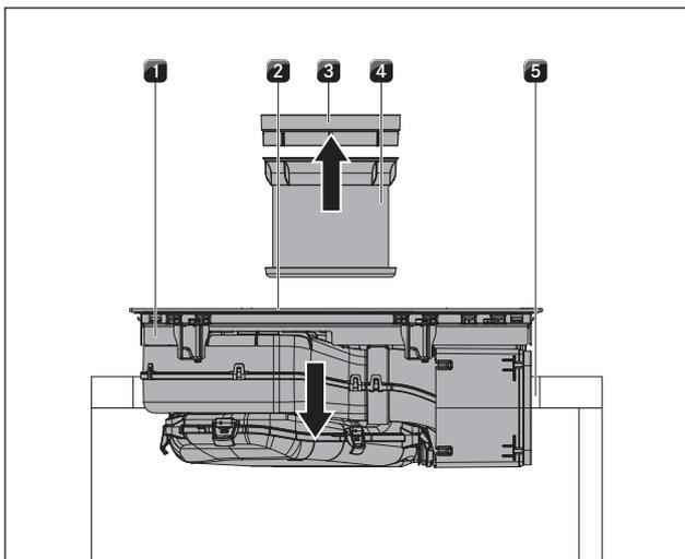
Fig. 6.14 Inserting the cooktop
