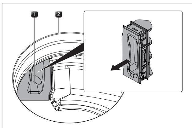
Fig. 6.19 Remove the filter replacement cover
