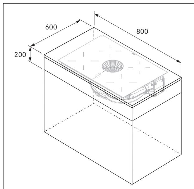
Fig. 6.2 Minimum unit dimensions
