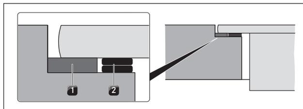
Fig. 6.16 Height adjustment plates
