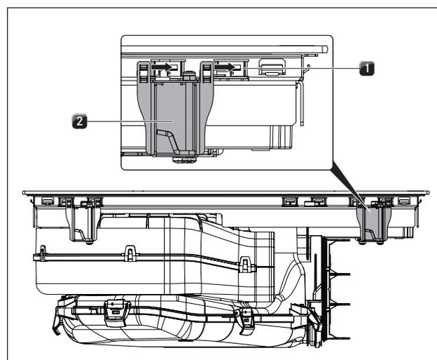
Fig. 6.27 Inserting the cooktop
