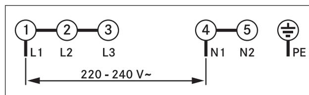
Fig. 6.35 Connection diagram 1-phase connection
