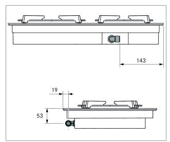
Fig. 4.45 Position of gas connection
