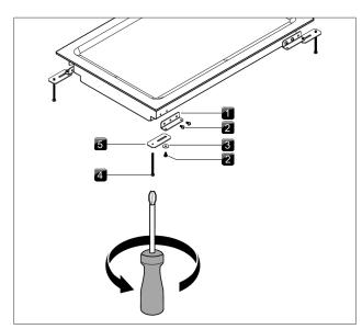
Fig. 4.32 Securing the Tepan stainless steel grill
