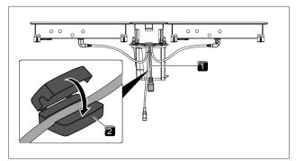
Fig. 4.40 Fitting split ferrite sleeves
