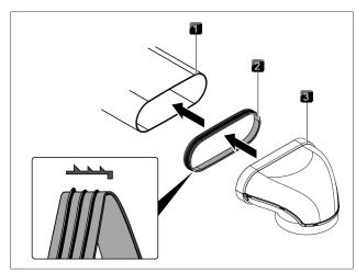
Fig. 4.26 Assembly of the duct system
