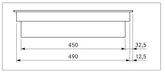
Fig. 3.13 CKIW device dimensions side view
