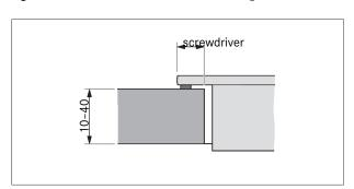
Fig. 4.13 Dimension of support for surface mounting
