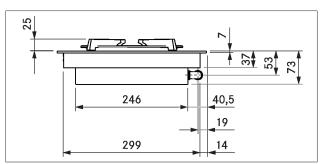
Fig. 3.21 CKG device dimensions front view
