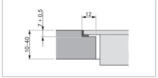
Fig. 4.11 Rebate dimensions for flush installation
