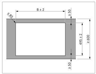
Fig. 4.12 Cut-out dimensions for surface mounting
