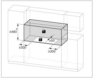
Fig. 4.3 Required clearance
