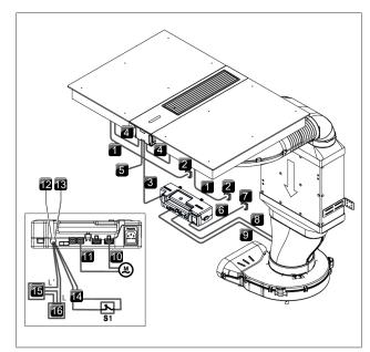
Fig. 4.38 Connection diagram for the cooktop extractor
