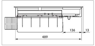
Fig. 3.3 CKA2/CKA2AB appliance dimensions side view
