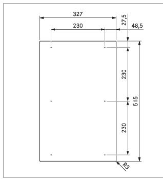
Fig. 3.5 CKFI device dimensions top view
