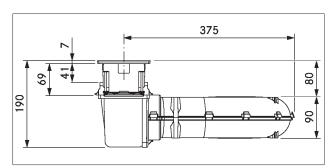
Fig. 3.2 CKA2/CKA2AB appliance dimensions front view
