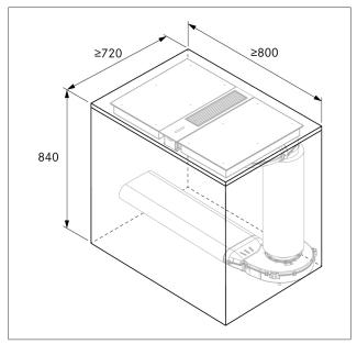
Fig. 4.15 Minimum installation dimensions with round silencer USDR50
