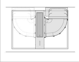
Fig. 4.19 Airflow towards the rear (right or left)
