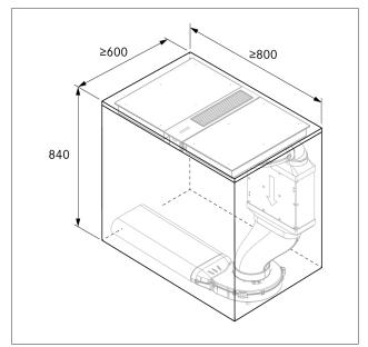
Fig. 4.14 Minimum installation dimensions with shallow silencer USDF
