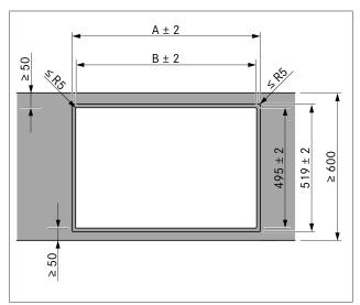
Fig. 4.10 Cut-out dimensions for flush installation
