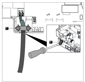
Fig. 4.36 Home-Out contacts with strain relief
