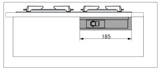
Fig. 4.8 Side cut-out for the gas connection
