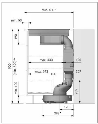
Fig. 4.16 Appliance installation dimensions with shallow silencer USDF, shallow duct connection EFV and offset transition piece EFRV110 (600 mm units)
