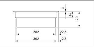
Fig. 3.12 CKIW device dimensions front view
