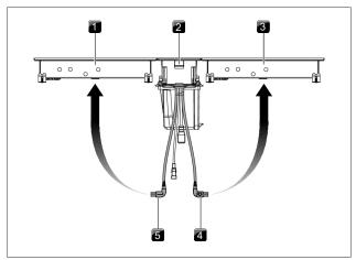
Fig. 4.39 Connecting the control cables to the cooktops
