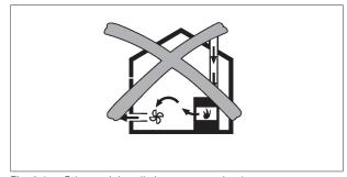
Fig. 4.1 Exhaust air installation - not permitted
