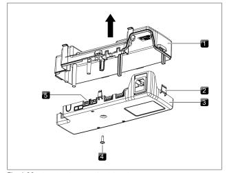
Fig. 4.33 Opening the control unit housing cover
