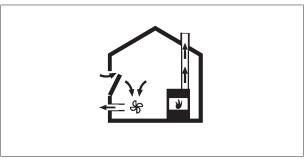
Fig. 4.2 Exhaust air installation - correct
