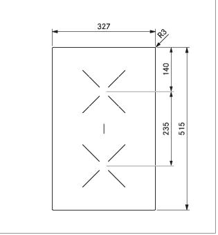
Fig. 3.17 CKCB device dimensions top view
