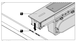
Fig. 4.24 Height adjustment plates for flush installation
