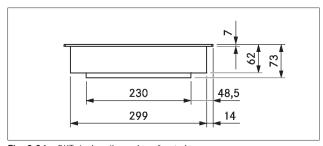
Fig. 3.24  $\,$  CKT device dimensions front view
