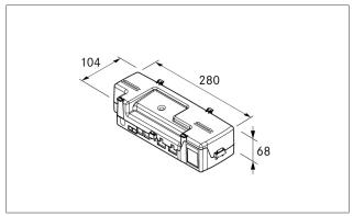
Fig. 3.4 Control unit dimensions
