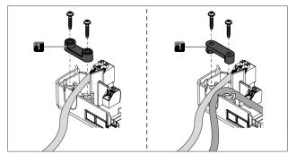
Fig. 4.37 Fitting the strain relief clamp
