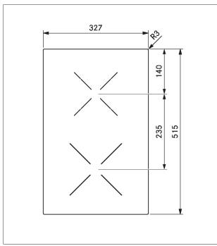
Fig. 3.14 CKCH device dimensions top view
