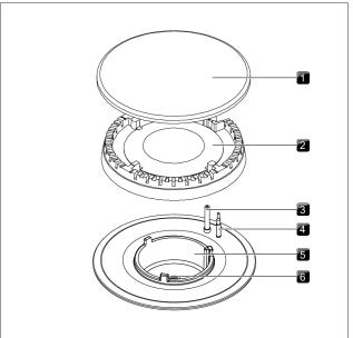
Fig. 4.46 Gas burner structure
