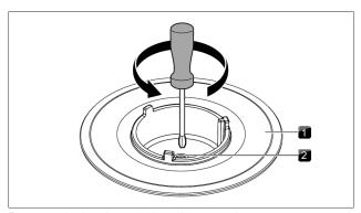
Fig. 4.47 Cooktop burner with gas burner nozzle
