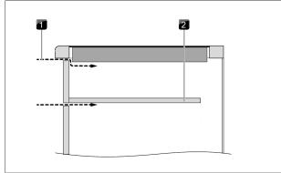
Fig. 4.6 Air supply at front of the unit
