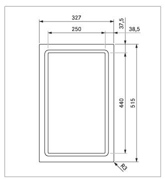
Fig. 3.23 CKT device dimensions top view
