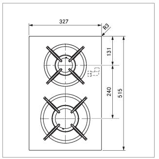
Fig. 3.20 CKG device dimensions top view
