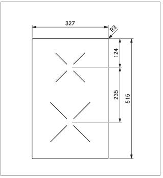
Fig. 3.8 CKI device dimensions top view
