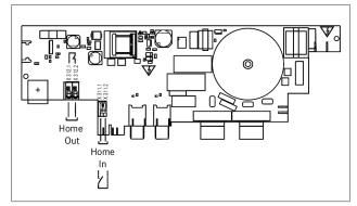
Fig. 4.35 Connection diagram for the external switch contacts
