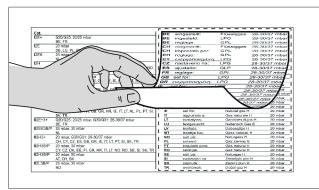
Fig. 4.48 Affixing the nozzle set nameplates
