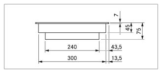
Fig. 3.18 CKCB device dimensions front view
