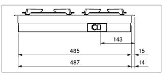
Fig. 3.22 CKG device dimensions side view
