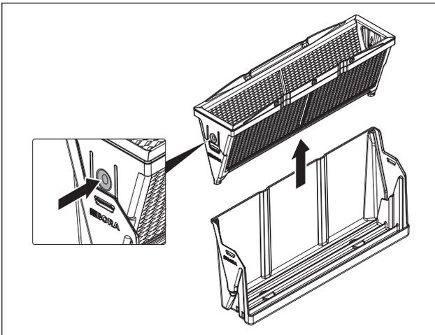
Fig. 9.3 Removing the grease filter
