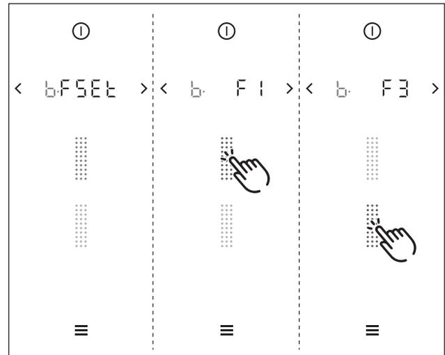
Fig. 7.13 Menu item B: Show filter type, change filter type and reset filter service life
