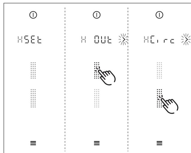
Fig. 5.1 Configuring the exhaust air system display
