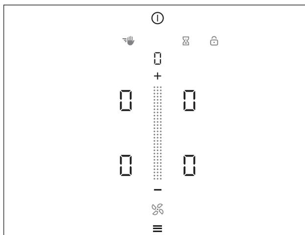
Fig. 6.1 Standard display after switching on
