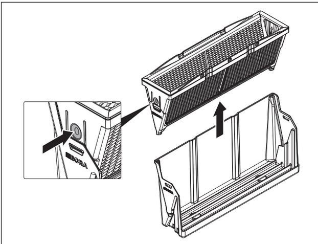
Fig. 9.3 Removing the grease filter
