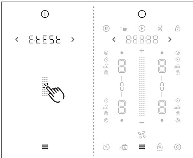
Fig. 8.4 Menu item E: Display and button test
