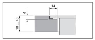
Fig. 5.4 Dimension of groove for flush installation
