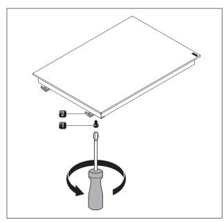
Fig. 5.16 Mounting brackets
