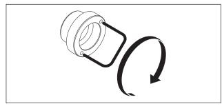
Fig. 5.11 Tighten the fixing nuts
