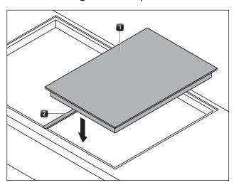
Fig. 5.14 Insert the mounting rail and cooktop
