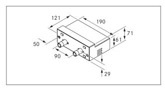
Fig. 3.2 Control box dimensions
