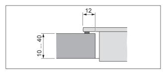
Fig. 5.6 Surface mounting cut
