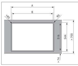
Fig. 5.3 Flush installation
