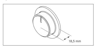
Fig. 5.13 Distance of the control knob
