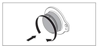
Fig. 6.1 Push and pull control knob
