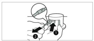
Fig. 6.2 How to pull out the vacuum hose coupling
