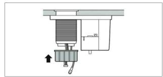
Fig. 8.16 Secure the appliance
