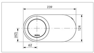
Fig. 3.2 QVac top view
