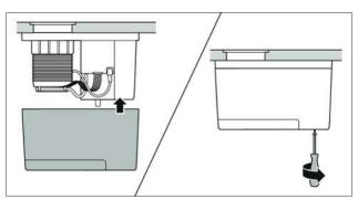
Fig. 8.19 Push the housing on and screw tight
