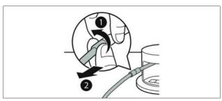
Fig. 6.3 How to remove the vacuum hose from the coupling
