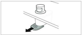
Fig. 6.5 How to pull out the drip tray
