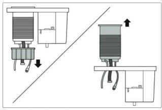
Fig. 8.12 How to disassemble the pop-up unit
