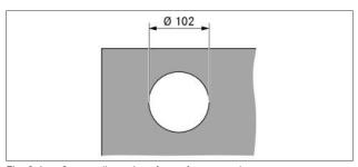
Fig. 8.4 Cut-out dimensions for surface mounting
