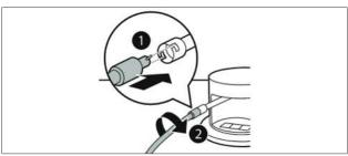
Fig. 6.4 How to attach the vacuum hose
