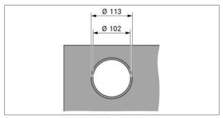
Fig. 8.6 Cut-out dimensions for flush installation
