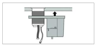
Fig. 8.15 Position the base unit
