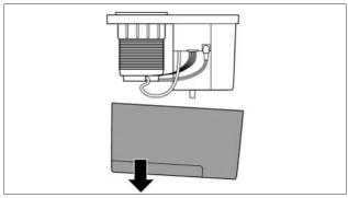
Fig. 8.10 Remove the housing
