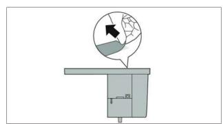
Fig. 8.14 Remove the film from the base unit
